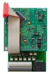
PCD2.T814: 33.6 kbps analogue modem (RS232 and TTL interface) PCD2.T851: ISDN-TA digital modem (RS232 and TTL interface)
